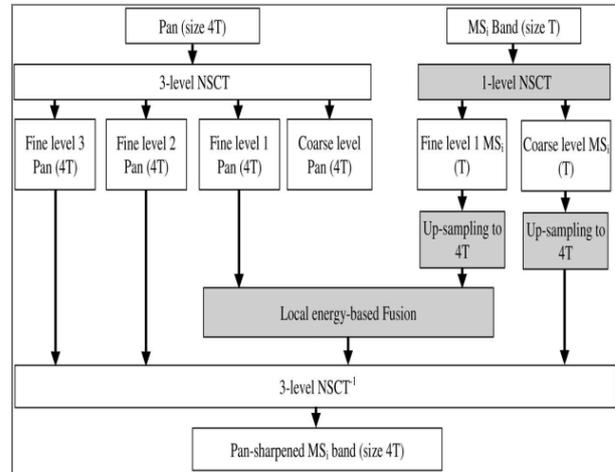
Fig.5 Existing Method based on Pan Sharpened Image.
